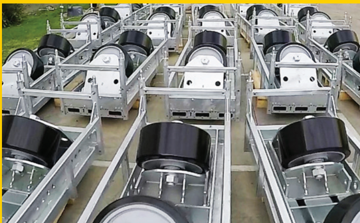
Supply of 150 30T pipe rollers for offshore oil & gas pipeline launch.
