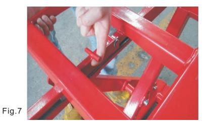
5. While holding both latches up and lift the top frame pass the latches until it is at its full, upper most position. Have the assistant hold the weight and insert the pivot pin in the hole in the base frame. See Fig. 8. With the Level Loader in this full upper most position the orange spring can be installed.
