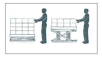
Fig. 20 Unloading Manually
