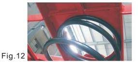
CORRECT Fully inserted into pocket
