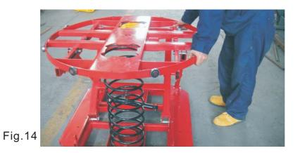
7. Remove the shock absorber pivot pin. Push down on top frame until latches engage. (Both latches will drop into place) .
