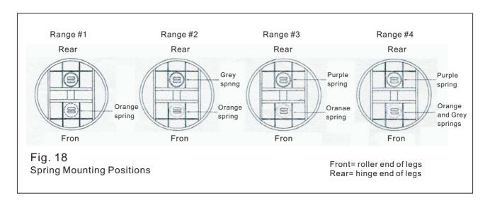
13. Figure 4 shows the position of additional springs if needed. Double-check to be sure you have the correct springs. Refer to Table I on page 7 and see that you have the correct springs for your application.
