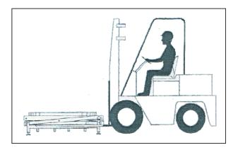
Fig. 23 Moving the Level Loader
