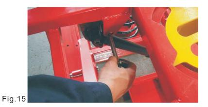
8. Reinstall the shock absorber pivot pin and linchpin.
