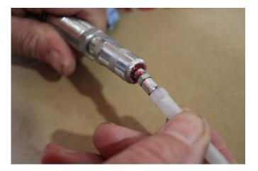
connect bottom of needle to hand operated grease gun hose. Best method is to position the ball end of the needle applicator at a slight angle and press firmly. STEP 2:
