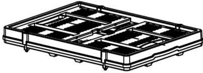
Collapsed KartR basket
