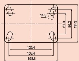
Baseplate dimensions & drilling patterns for Kingpinless Castors
