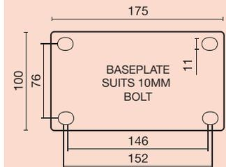
Baseplate dimensions & drilling patterns for 1000 Series Castors
