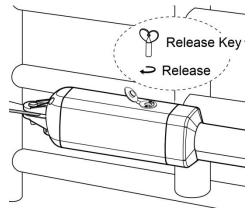
opener is level. While holding the gate opener in the level position, temporarily secure it with two C-clamps.
