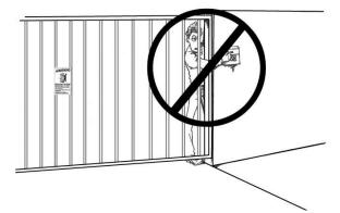
11. Controls intended to be used to reset an operator after 2 sequential activations of the entrapment protection device or devices must be located in the line of sight of the gate, or easily accessible controls shall have a security feature to prevent unauthorized use. Never allow anyone to hang on or ride the gate during the entire travel of the gate.
