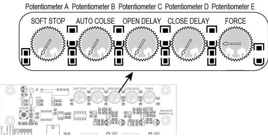
**Potentiometer A** is used to adjust the soft stop period of the gate opener. Turn the potentiometer clockwise to increase the soft stop period, and turn it counter-clockwise to decrease the soft stop period. The soft stop period can be adjusted steplessly from 1 to 5 seconds.
