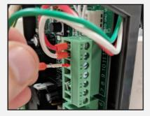
Insert the wire into the number on the terminal that you are looking to connect to. Refer to Pages 20 & 21
