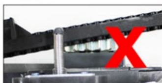
Gear rack misaligned. Do not attempt to use if misaligned.
