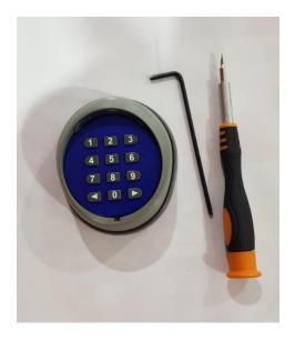
Using a small flat blade screwdriver, remove the blue front panel from the keypad.
