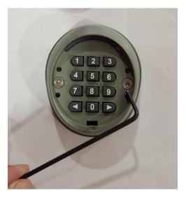
After screws are removed, lift the housing. The rear plate should drop away.
