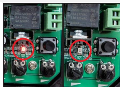
The Learn LED will flash repeatedly and then turn OFF. when the remote is paired.
