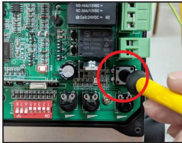
Press and hold the learn button (S1) until the Learn LED flashes ON.
