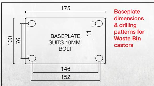
Baseplate dimensions & drilling patterns for Waste Bin castors
