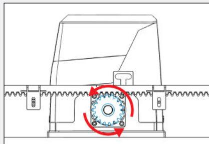
The motor cog will turn counter-clockwise, moving the gate frame.
