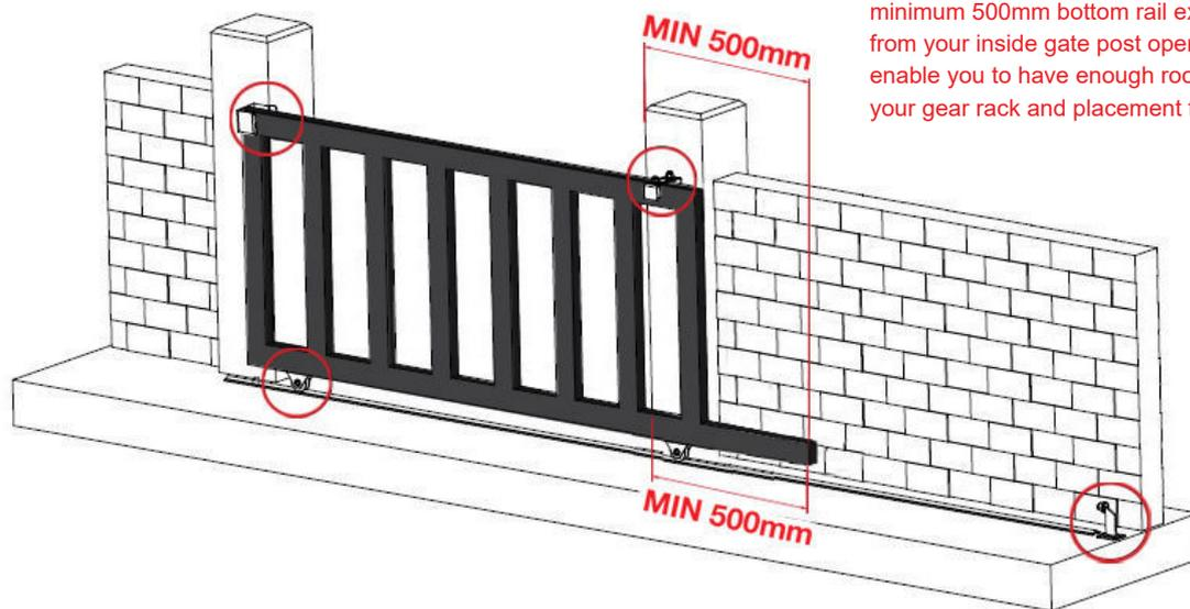
It is recommended that you allow a minimum 500mm bottom rail extension from your inside gate post opening. This will enable you to have enough room to secure your gear rack and placement for the motor.
